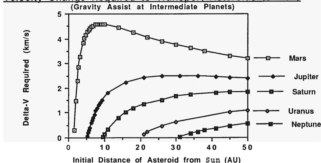
Fig.10 Using gravity assists, the  $\Delta V$  required to propel an outer solar system asteroid onto a collision course with Mars can be less than 0.5 km/s. Such "falling" objects can release much more energy upon impact than was required to set them in motion.
