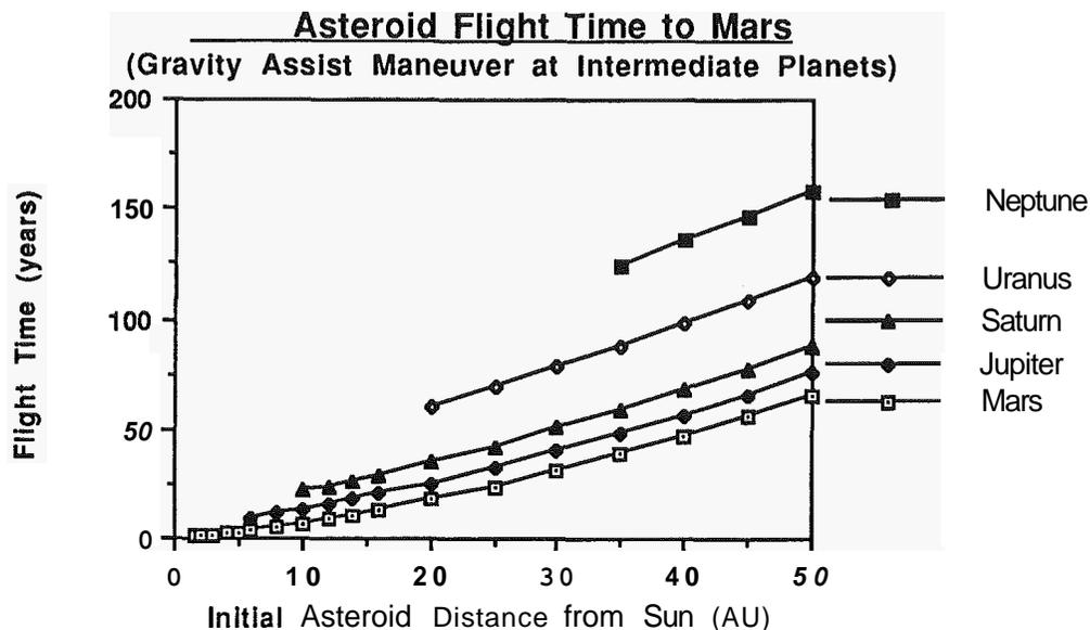
Fig.II Ballistic flight times from the outer solar system to Mars are typically between 25 and 50 years.
