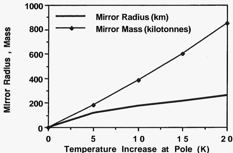
Fig.9. Solar sail mirrors with radii on the order of 100 km and masses of 200,000 tonnes can produce the 5 K temperature rise required to vaporize the CO<sub>2</sub> in Mars' south polar cap. It may be possible to construct such mirrors in space
