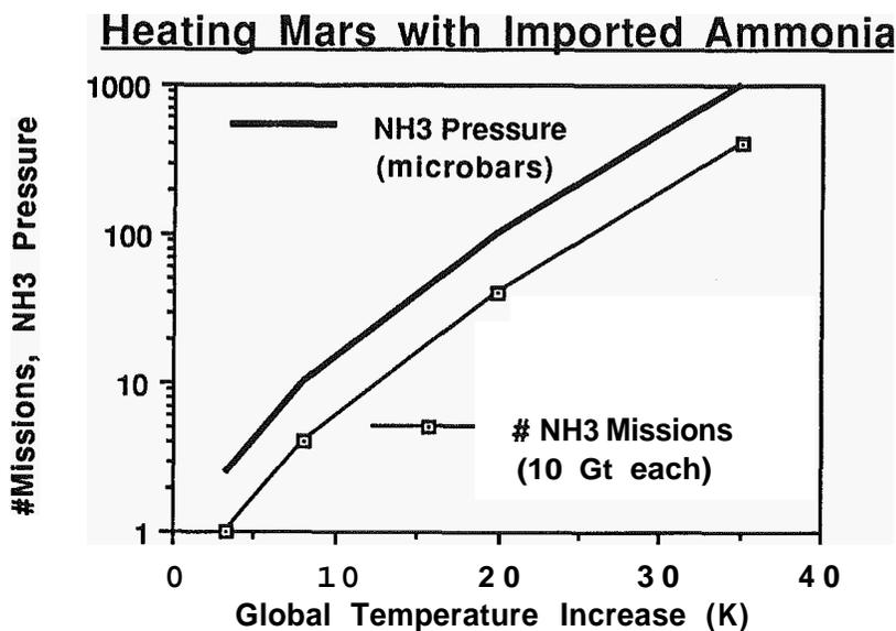
Fig. 12 Importing four 10 billion tonne ammonia asteroids to Mars would impose an 8 K temperature rise, which after amplification by CO<sub>2</sub> feedback could create drastic changes in global conditions.
