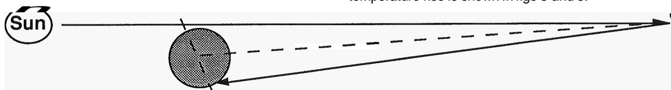
Fig.8 Solar sails of 4 tonnes/km<sup>2</sup> density can be held stationary above Mars by light pressure at an altitude of 214,000 km. Wasting a small amount of light allows shadowing to be avoided.
